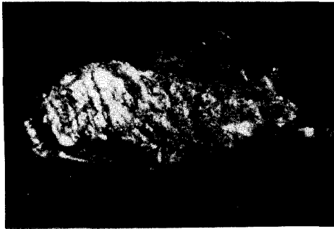
Fig. 22. Fractography showing beach mark(35 x).
