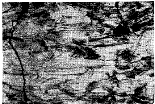
Fig. 25. Etched surface showing transgranular crack propagation(80x).
