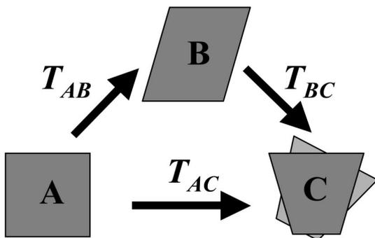
**Fig 8.** Use of consistency to estimate registration errors. Given three independently acquired images (A,B,C), registration of A with C can be achieved either by first transforming A to B ( $T_{AB}$ ), followed by transformation from B to C ( $T_{BC}$ ), or by direct transformation from A to C ( $T_{AC}$ ). The two transformations ( $T_{AB}T_{BC}$ ) and  $T_{AC}$  should be identical. The residual difference can be attributed to errors in each of the transformations.
