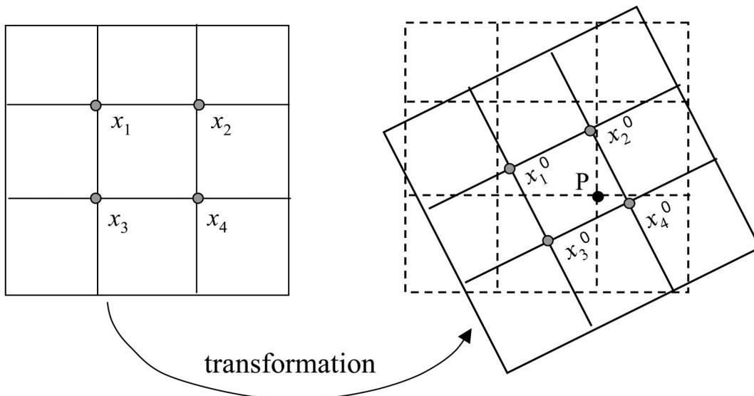
**Fig 6. Interpolation associated with image registration.** The transformation of an image results in the re-mapping of each voxel to a new location. For the purpose of registration, the transformed image must be re-sampled on the original grid. Determination of the intensity at each original grid point (for example point P) requires estimation based on surrounding voxel values. The resulting interpolation will result in some degree of smoothing of the original image.
