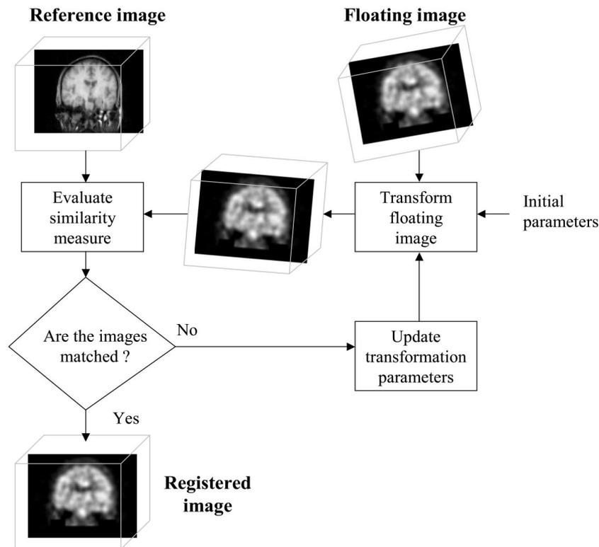
**Fig 1. Schematic of a general image registration algorithm. An initial set of transformation parameters is applied to the floating image. The transformed floating image is then compared with the reference image by assessing the similarity between the two images. The algorithm iteratively updates the transformation parameters and reassesses the similarity measure until alignment is achieved.**
