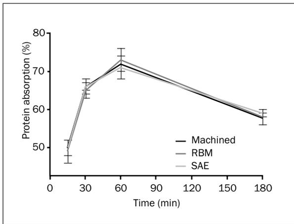
**Fig 3** Absorption of bovine serum albumin to titanium surfaces. Error bars are standard error of the mean.
