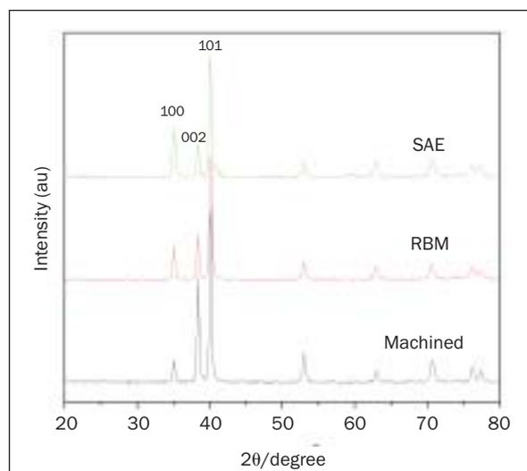
**Fig 2** XRD patterns. All peaks are assigned to alpha-titanium.
