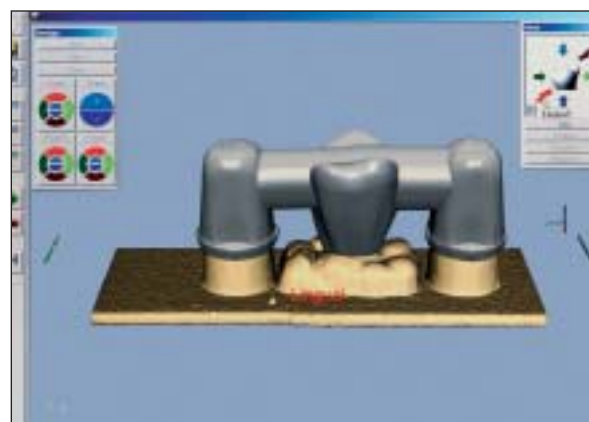
Fig 2 Screenshot displaying a typical FPD frame designed on the basis of an optical impression.
