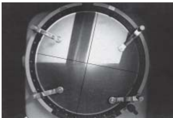
Fig 3 Nikon Profile projector and master cast specimen for readings.
