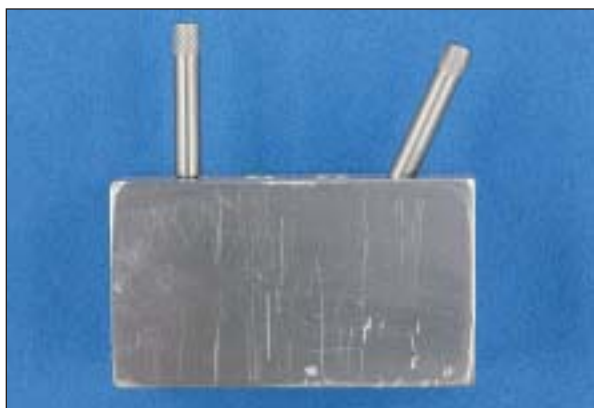
Fig 1 Metal matrix with 1 implant at a 90-degree angle and the other at a 65-degree angle in relation to the surface.
