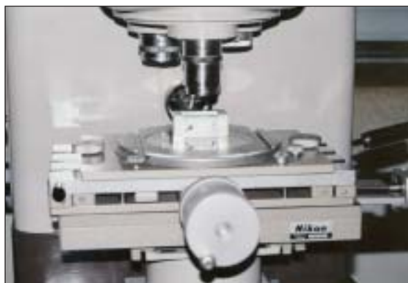
Fig 4 View of graduated profilometer screen and angulation of a referential element in relation to the x axis.
