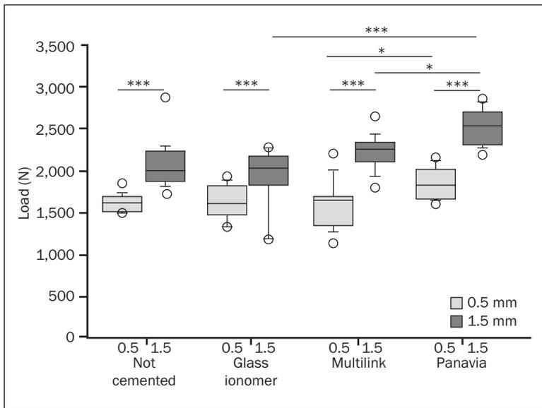
**Fig 5** Fracture loads (n = 15) of esthetic ceramic CAD/CAM crowns with 0.5 and 1.5 mm occlusal thickness on zirconia abutments \**P* < .05, \*\**P* < .01, \*\*\**P* < .001; Scheffé tests.
