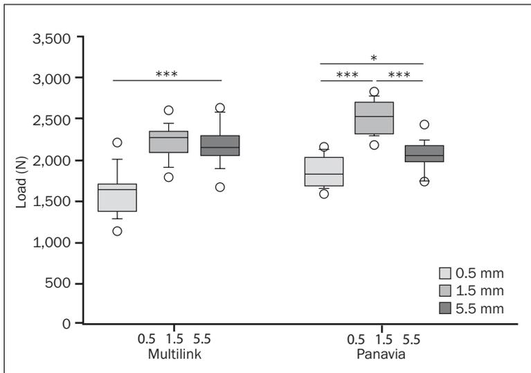
**Fig 6** Fracture loads (n = 15) of esthetic ceramic CAD/CAM crowns with 0.5 and 1.5 mm occlusal thicknesses on standard zirconia abutments (2) and with 5.5 mm occlusal thickness on shortened (3) zirconia abutments. All crowns seated with adhesive cements c and d. \**P* < .05, \*\*\**P* < .001; Scheffé tests.
