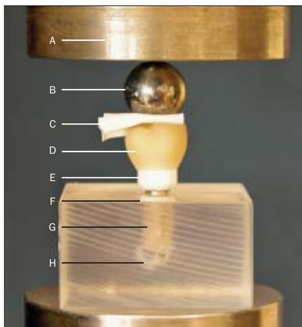
**Fig 3** Loading until fracture: (A) loading stamp, (B) steel ball, (C) Teflon foil, (D) sample crown, (E) abutment, (F) fixture, (G) implant, (H) polymethyl methacrylate supporting block.
