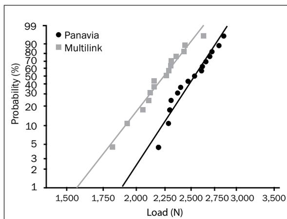
**Fig 8** Probability plot for failure of esthetic ceramic CAD/CAM-generated crowns with 1.5-mm occlusal thickness placed with adhesive cements c (Multilink) and d (Panavia) on zirconia implant abutments. The steepness of the lines indicates the range of dependability. The steepness of the line is a measure for the dependability of the material.<sup>30</sup>
