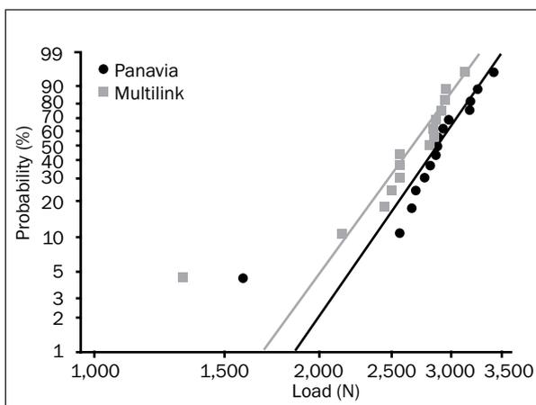
**Fig 7** Probability plot for failure of esthetic ceramic CAD/CAM-generated crowns with 1.5-mm occlusal thickness placed with adhesive cements c (Multilink) and d (Panavia) on titanium implant abutments. The lowest value for Multilink was related to a sample crown showing a hairline crack before loading. The lowest value for Panavia was related to a chipping fracture. The steepness of the line is a measure for the dependability of the material.<sup>30</sup>
