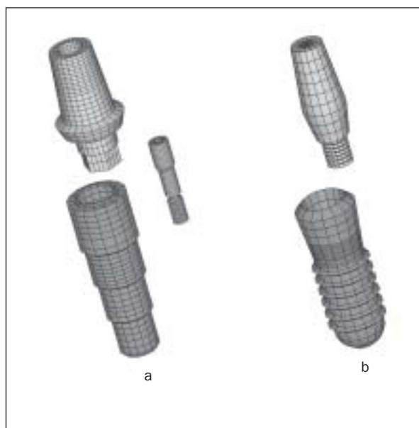
**Fig 2** 3D FEA models of an implant-supported prosthesis constructed for this study. (a) Frialit-2 (FRI) system, including the abutment, abutment screw, and implant. (b) Straumann (STR) system, including the abutment and implant.
