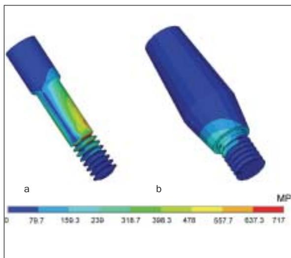
**Fig 6** Stress concentration regions of the (a) Frialit-2 (FRI) abutment screw and (b) the Straumann (STR) solid abutment.
