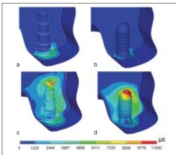
**Fig 5** Strain distributions of (a) the Frialit-2 (FRI) implant system and (b) the Straumann (STR) implant system placed in position 1 with bone type 1 and applied lateral forces. Maximum strain is concentrated at the cervical regions in cortical bone. (c and d) The same systems placed in position 1 with bone type 4 and applied lateral forces. Here, maximum strain is concentrated in cancellous bone at the implant apex.
