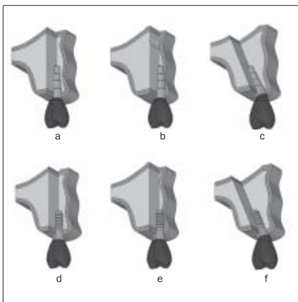
**Fig 1** Six solid models showing 2 implant systems, Frialit-2 and Straumann, in 3 positions with fabricated crowns: (a) a Frialit-2 implant in position 1 (FRI; P1); (b) a Frialit-2 implant in position 2 (FRI; P2); (c) a Frialit-2 implant in position P3 (FRI; P3); (d) a Straumann implant in position 1 (STR; P1); (e) a Straumann implant in position 2 (STR; P2); and (f) a Straumann implant in position 3 (STR; P3).
