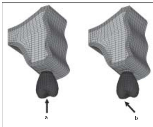
entirely homogeneous compact bone, (2) 1.5-mm layer of cortical bone bounding a core of dense cancellous bone, (3) 0.75-mm layer of cortical bone bounding a core of dense cancellous bone, and (4) 0.75-mm layer of cortical bone bounding a core of low-density cancellous bone. Elastic properties used for bone and restorative materials were obtained from the literature (Table 2).
