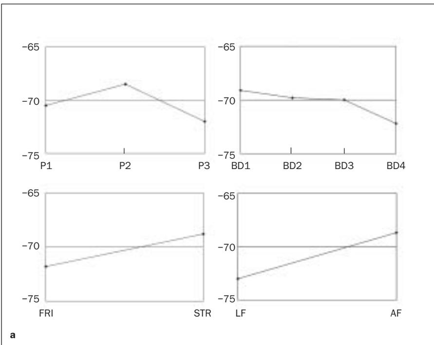
**Fig 4** Main effects of implant position (P1, P2, or P3), bone density (1 to 4), implant type (STR or FRI), and loading condition (AF or LF) at each level for transformed maximum von Mises strain on (a) cortical bone, (b, facing page) cancellous bone, and (c, facing page) transformed maximum von Mises stress on the implant.
