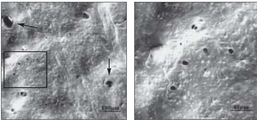
**Fig 2** Scanning electron photomicrograph of a membrane. (a) Several small pores (boxed area) and large pores (arrows) on the membrane surface. (b) Detail of the small pores.
