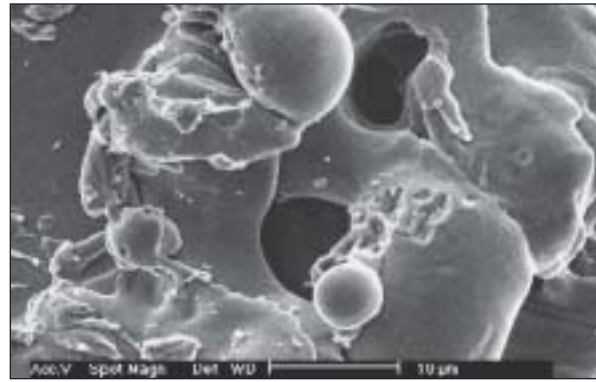
Fig 2 Surface morphology of titanium implants. (a) Low-magnification image and (b) high-magnification image.
