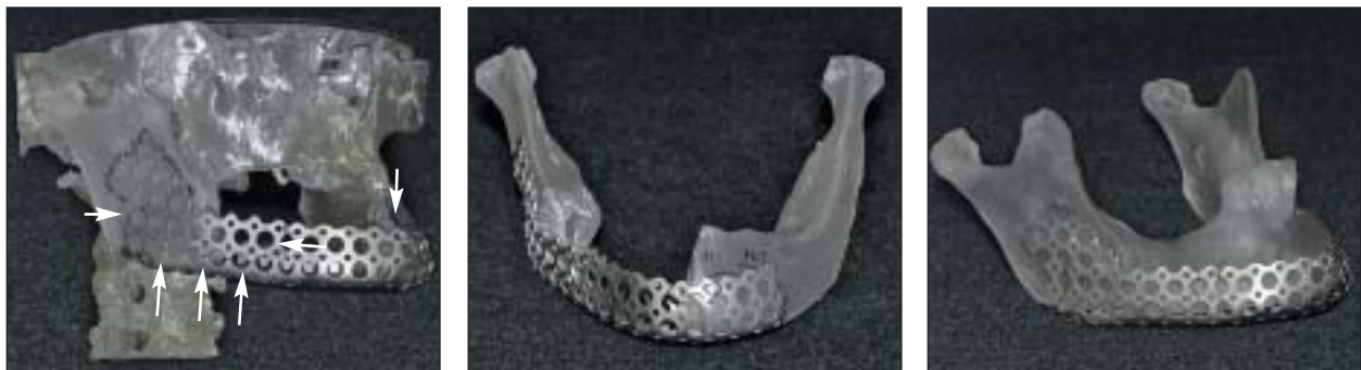
Fig 2 Reinforced titanium mesh shaped to match the model with a segmental defect. (Arrows, areas reinforced by laser welding.)
