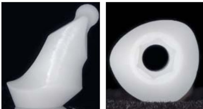
Fig 1 Atlantis abutment in zirconia test sample ( left: lateral view; right: interface ).
