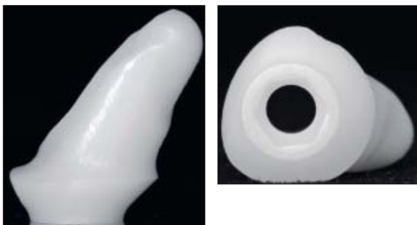
Fig 2 Nobel Biocare Procera AllZirkon abutment test sample ( left: lateral view; right: interface ).
