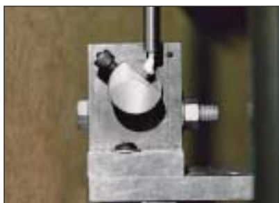
Fig 3 Zirconia abutment mounted in test apparatus at 40-degree angle to the applied load.
