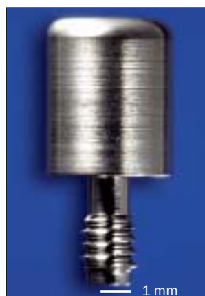
Fig 2 After an initial submerged healing interval, each implant was exposed and connected to a straight-sided abutment with a length of 5 mm and a diameter of 4.1 mm to effect some loading.
