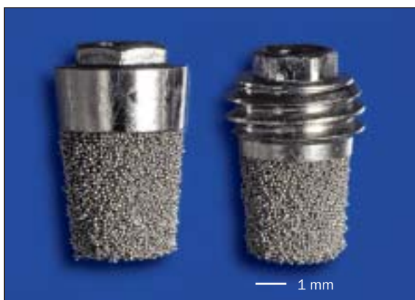
Fig 1 The control and hybrid implants; the hybrid implant had 3 coronal threads.
