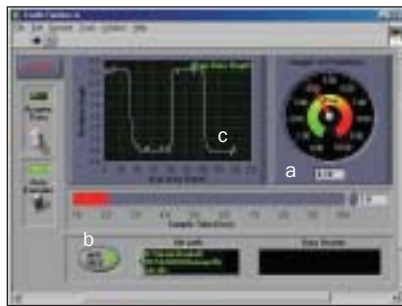
Fig 3 Software interface (VI) on computer screen showing (a) the angle of rotation (degrees), (b) the sample time (seconds), and (c) a raw data graph showing clockwise (downward) and counterclockwise (upward) rotation of abutment.
