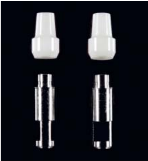
Fig 1 Industrially manufactured titanium abutments modified for the test setup and the industrially manufactured zirconia ceramic copings. The height of the titanium abutments was 2.7 mm. Abutment diameter was 2.86 mm in groups ALC30 and ABR30 and 2.80 mm in groups ALC60 and ABR60.
