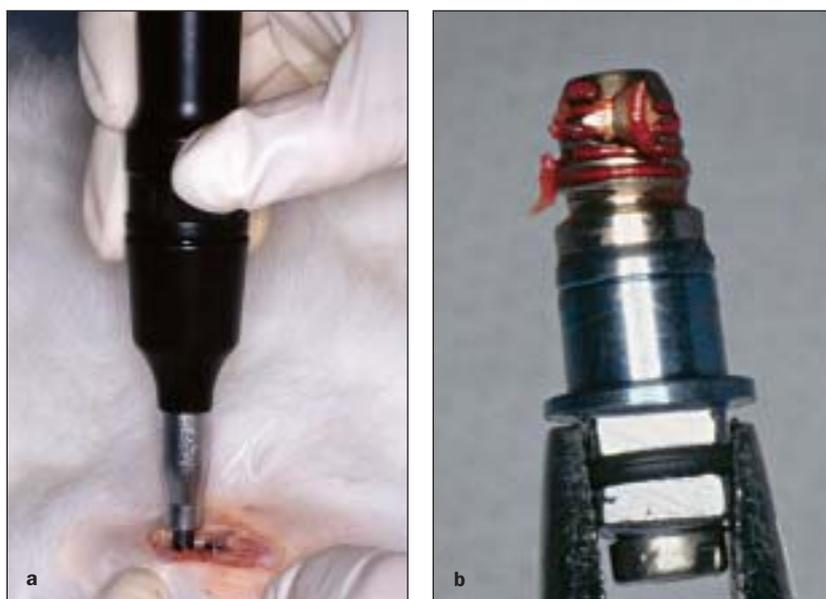
**Fig 2** (a) Removal torque test. (b) Acid-etched implant after removal torque test. Some bone chips were attached to the implant surface.
