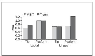
**Fig 4** Mean labial and lingual deviations after transmucosal implantation with the VISIT and the StealthStation Treon navigation systems.
