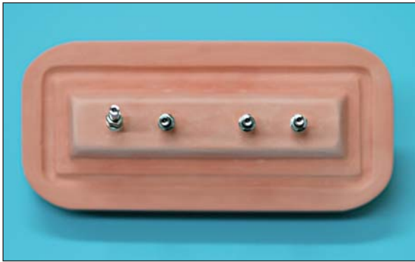
Fig 1 Superior view of the master model with 4 internal-connection implant replicas. Square impression copings were connected to show the angulation of the replicas. The pair on the left represents the divergent condition, and the pair on the right represents the parallel condition.
