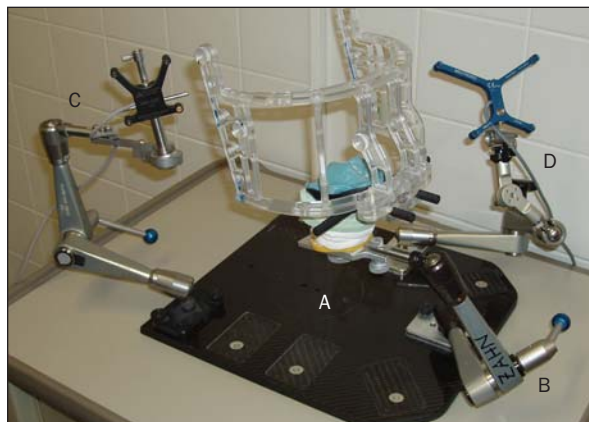
Fig 2 Laboratory setup for registration and navigation: A = base plate; B = mechanical arm for the fixation of the dental stone cast by the dental articulator's fixation system; C = EasyTaxis aiming device; D = reference arc. For registration, the mouthpiece with the registration frame attached was mounted to the fixed dental stone cast. By touching the registration markers with the navigation probe, the "virtual" (CT-data) markers were linked to the corresponding "real" (setup) markers, which allowed the transfer of the 3D surgical plan to the dental stone cast.
