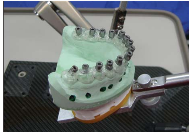
Fig 3 Method 1 (direct bur tube positioning). (Left) The aiming device of the navigation system was used for direct positioning of 2-mm surgical bur tubes on the dental stone casts. One by one, the bur tubes were affixed into a prefabricated template with blue light-curing resin. (Right) Finished surgical template on one of the mandibular casts.
