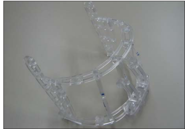
Fig 1 Modified Vogele-Bale-Hohner (VBH) mouthpiece (Medical Intelligence, Schwabmuenchen, Germany) and reference frame. (Left) The mouthpiece (A) was loaded with the dental impressions of the maxillary and mandibular casts, which were mounted to the dental articulator. (Right) The u-shaped registration frame included 7 spherical registration markers (glass, diameter 5.8 mm) broadly distributed around the region of interest and could be mounted to the anterior extensions of the mouthpiece.
