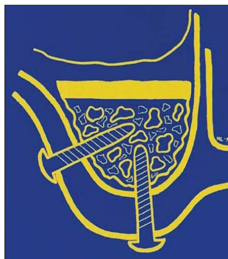
Fig 2 Fig 2 Two-stage surgery; technique where bone graft is fixed with osteosynthesis screws.
