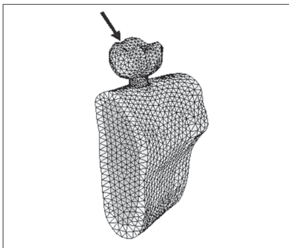
Fig 1 The finite element model included the crown, the implant, and the posterior mandible. The model contains about 42,500 elements and 61,300 nodes. The 100-N oblique load was applied to the buccal cusp of the crown. The boundary condition was set to fix the bottom surface of the mandibular section.
