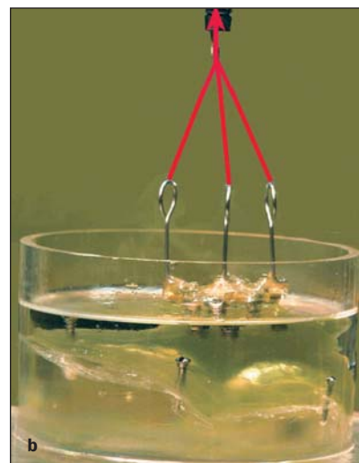
Fig 6 Test setup for determination of stress during removal. (a) Perpendicular to axes of implants. (b) Parallel to axes of implants.
