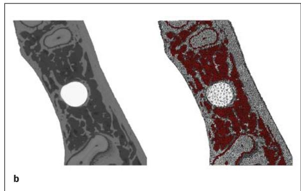
**Fig 3** 3D volume rendering of sample 4-UR obtained from  $\mu$ CT scanning (3a, left) and its corresponding FE model (3a, right). A single-slice scan of sample 1-LL (3b, left) and the corresponding section from the FE model (3b, right) are also presented. The  $\mu$ CT 3D rendering of sample 3-LR (3c, left) is presented with the corresponding FE where only the bone is depicted (3c, right).
