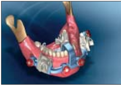
Fig 1 The intraoral device, which consists of a rigid frame ( blue ) to which affixation pins are attached ( red ), and in which tactile sensors containing needle arrays are affixed ( gray ).
