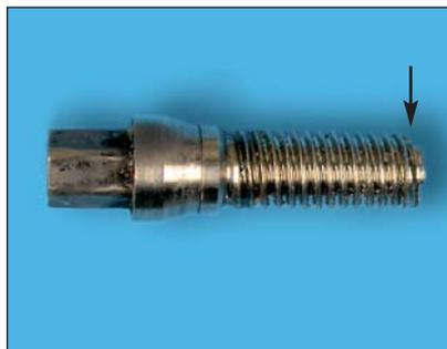
**Fig 5a** Fractured implant (sample R/0/1). The fracture occurred at the level of the start of the self-tapping notch (arrow).
