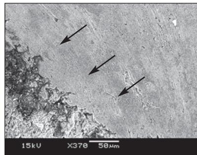
**Fig 5c** Boxed area of Fig 5b at a higher magnification showing fatigue striations (arrows), indicating fatigue failure.
