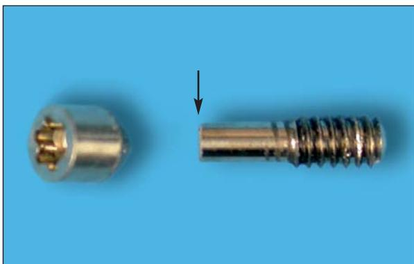
**Fig 3** Failed abutment screw (sample N+/3) at the junction of the screw head and the screw shank (arrow).
