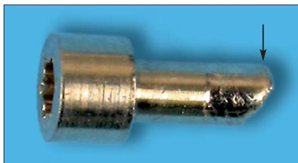
**Fig 4** Failed abutment screw (sample R-/5) at the first thread (arrow).
