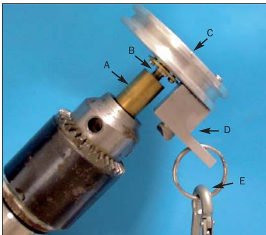
**Fig 1** Profile view of the assembled test specimen setup. (a) Implant holder, (b) implant specimen, (c) bearing housing, (d) L-bracket, and (e) applied load.
