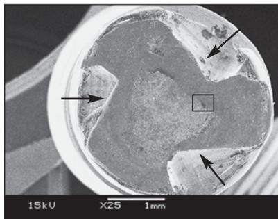
**Fig 5b** The surface of fractured implant R/0/1 under SEM. Fracture occurred at the start of the self-tapping notch (arrows).
