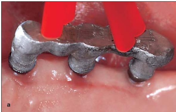
Fig 2 In vivo measurement of cementable FPDs. (a) FPD with strain gauges fixed on the pontics (SG-pAB and SG-pBC) placed on the abutments. (b) Strain gauge signals from SG-pAB and SG-pBC during the cementation procedure at different time points: (1) SGs set to zero; (2) maximum bite force applied; (3) force reduced and sustained for 3 minutes; (4) FPD relieved; and (5) final strain values recorded for analysis.
