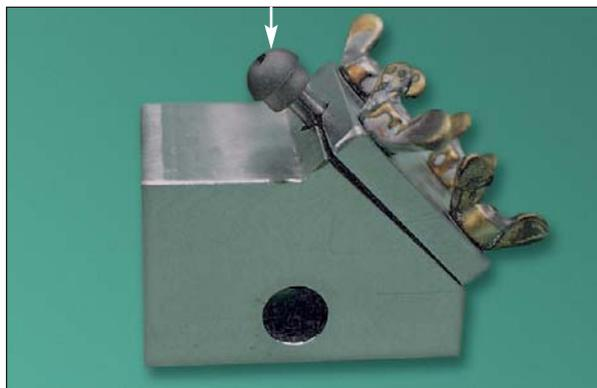
**Fig 2** The test apparatus with the test specimen at a 30-degree angle. The arrow indicates the load direction.
