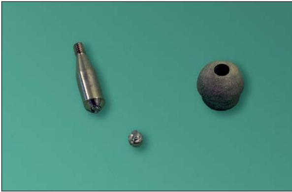
**Fig 4** Typical failed specimen from the 45-degree abutment group.
