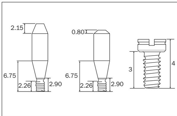
**Fig 1** The shape of the abutments tested. The shape of the retaining screw, exaggerated, is also shown.
