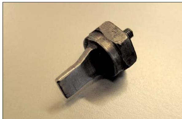
**Fig 3** Crosshead design with a rounded edge of 1 mm in diameter.
