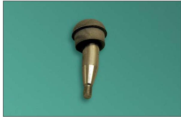
**Fig 5** Typical failed specimen from the 20-degree abutment group.
