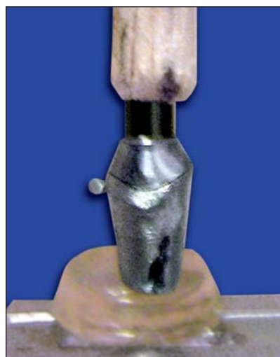
Fig 5 Specimen assembly used to stabilize the coping on the die during the measurement procedure on the microscope stage.
