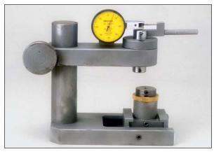
**Fig 2** Custom-made apparatus used to assess rotational freedom at the implant-abutment interface. The needle pointer, with its clockwise and counterclockwise rotation, allowed rotational freedom to be recorded.
