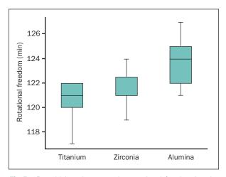
**Fig 5** Box-whisker plot comparing rotational freedom in minutes for each material. Top and bottom of boxes show 75th and 25th percentiles. Top and bottom of whiskers depict maximum and minimum values. The horizontal line inside the boxes is the median value.
