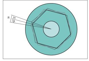
Fig 3 Diagram illustrating rotational freedom (R) between the hexagonal extension of the implant and Procera abutment counterpart. R represents difference between clockwise ( $\alpha$ ) and counterclockwise ( $\beta$ ) rotation of the needle pointer attached to the Procera abutment collar.
