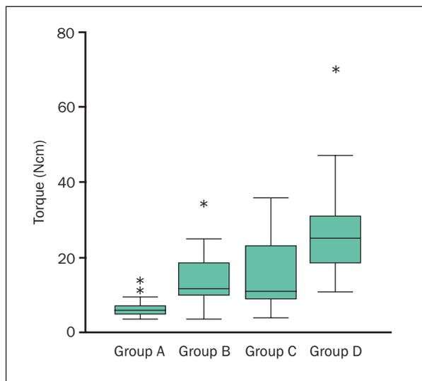
**Fig 3** Torque moment values following standard and under-dimensioned drilling.
