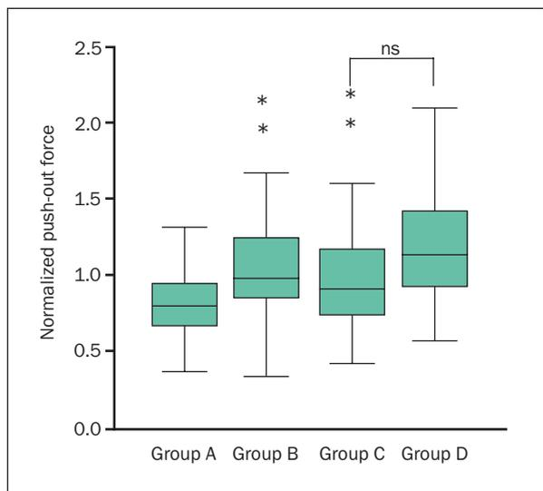
**Fig 7** Normalized push-out force values following standard and under-dimensioned drilling.
