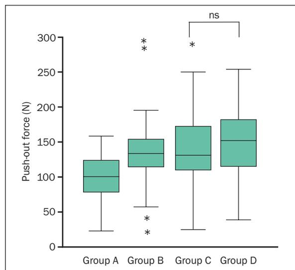
**Fig 6** Push-out force values following standard and under-dimensioned drilling.
