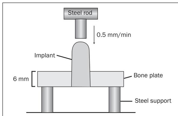
**Fig 2** Experimental setup for the push-out testing.
