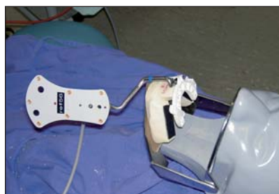
Fig 3 The mandible model was mounted to a phantom head to simulate clinical situation. The locating horseshoe element was cemented onto the anterior segment of the model base and was connected by a metallic pole to a reference body for tracking purposes. The handpiece and the reference body must remain within the area of the tracking camera. They must face the tracking camera to ensure constant tracking for surgical navigation.
