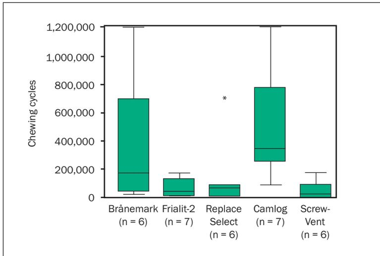
**Fig 3** Box-plot diagram of recorded chewing cycles until bacterial penetration occurred. Asterisk depicts an extreme value for Replace select specimen no. 7. The boxes represent the first and third quartiles of the recorded chewing cycles; the line, the medians.
