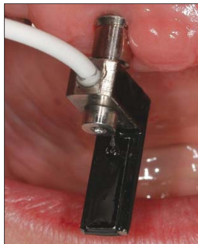
Fig 1 (Right) Intraoral view of RFA measuring device (Osstell) mounted to a Straumann implant with the octa-abutment in situ.
