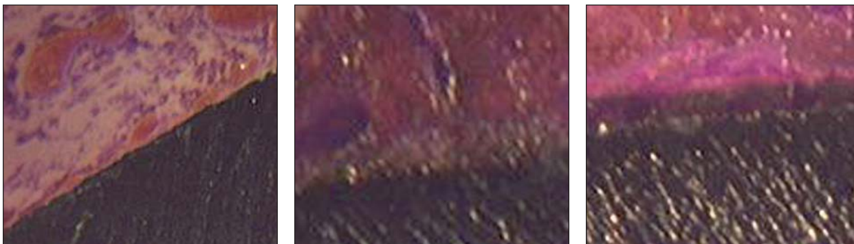
Fig 2 Histology of (a) titanium controls, (b) plasma-sprayed HA-coated implants, and (c) HA-coated implants created using SPA after 3 weeks of implantation (original magnification \times 40 ).
