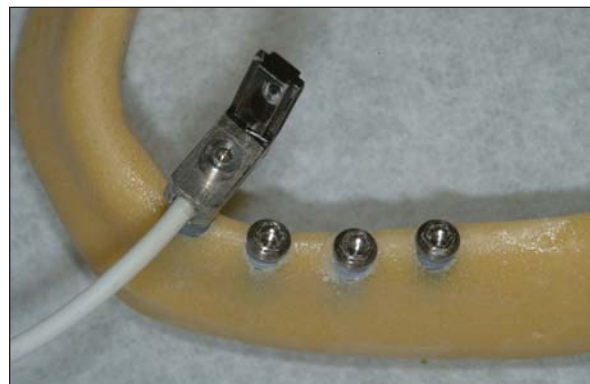
Fig 1b An Osstell transducer attached to an RP Brånemark System implant perpendicular to the alveolar ridge of a synthetic bone model.
