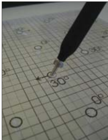
Fig 2b The tip of the 3D-digitizer probe was specifically designed to precisely fit in the 1.7-mm-wide bur holes.
