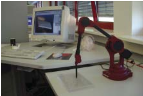
Fig 2a A high resolution 3D-digitizer probe ( right ) was used to detect the coordinates of the drilled holes. The 3D-digitizer was connected to a computer workstation. The data was converted to and analyzed by a computer-aided design (CAD) system ( left ).
