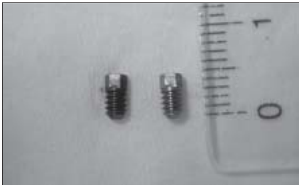
Fig 1 The experimental samples after toluidine blue staining. The collagen-coated titanium (coTi) screw (left) absorbed the dye and shows homogenous staining.
