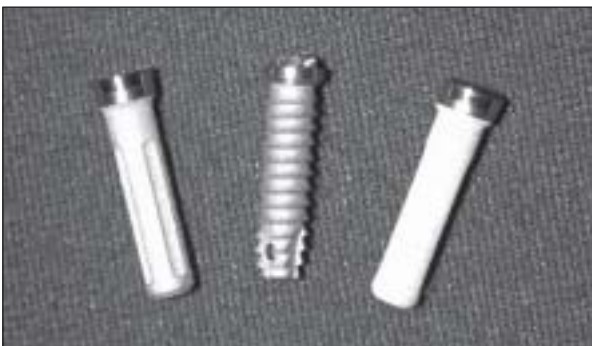
Fig 1 The 3 types of BioloK implants used were (left to right) titanium cylinder, titanium screw, and HA-coated cylinder.
