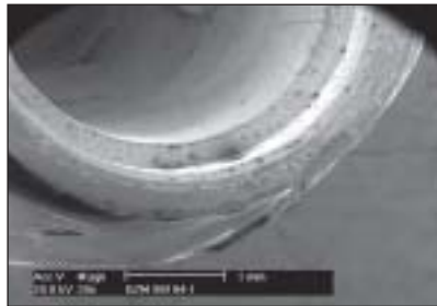
Fig 3 Scanning electron micrographs of the corroded crowns and implants.
