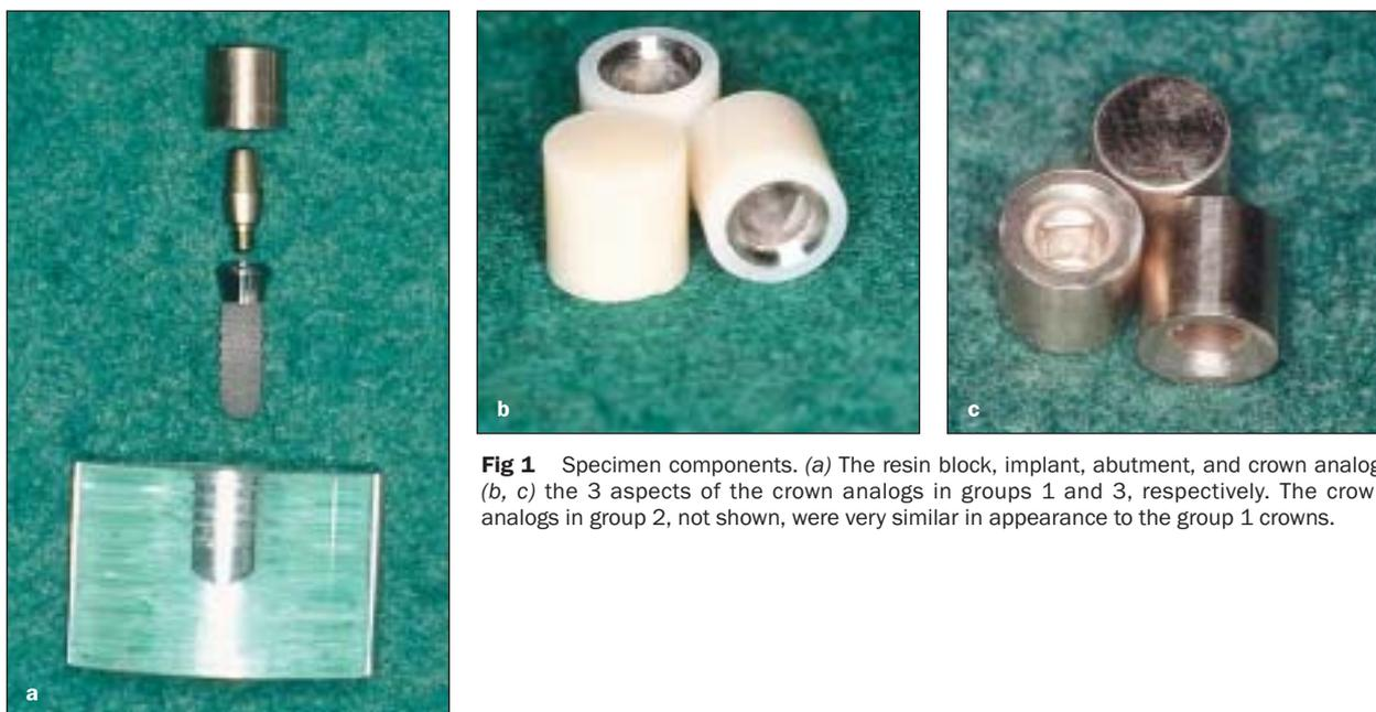
**Fig 1** Specimen components. (a) The resin block, implant, abutment, and crown analog; (b, c) the 3 aspects of the crown analogs in groups 1 and 3, respectively. The crown analogs in group 2, not shown, were very similar in appearance to the group 1 crowns.
