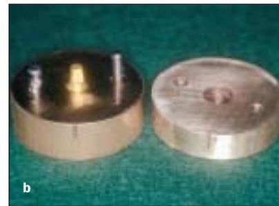
**Fig 4** (a) The crown-forming jig and crown analogs from groups 1 and 2 and (b) the jig for group 3. The implant analog was placed in the lower block of each jig.
