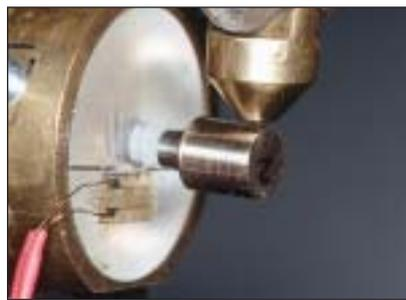
**Fig 5** Specimen mounted in the holder of the lever-type testing machine. The moisture sealing tape had not yet been applied over the strain gauge.
