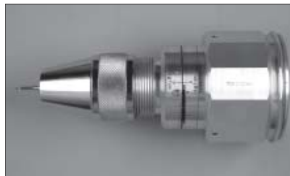
Fig 2 Mechanical torque gauge (model 6 BTG, Tohnichi Manufacturing, Tokyo, Japan) with the selected driver tip.
