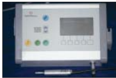
Fig 1d (Left) A TiUnite implant connected to the Osstell equipment by a transducer for resonance frequency evaluation.
