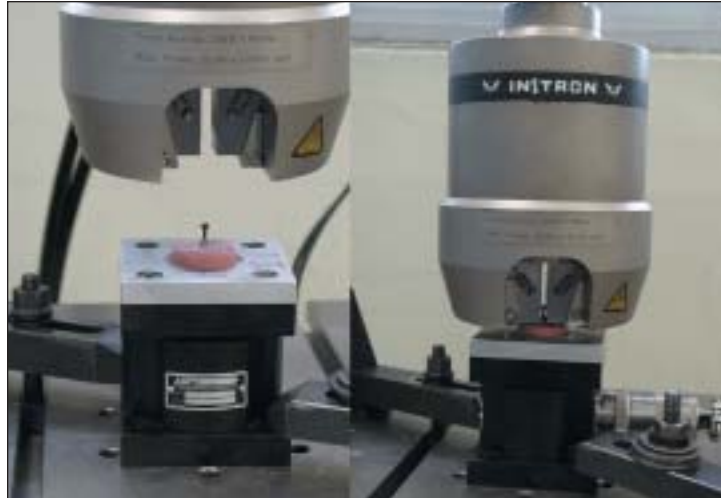
Fig 1b (Below) The specimen mounting plate was fixed on the load cell. The axial screw on top of the implant was used to stabilize the axis of the implant and to allow the test machine to get enough grip and fixation.
