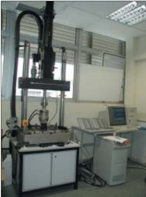
Fig 1a (Left) The RTVs were collected with an Instron tension-torsion system using an axial-torsional load cell.
