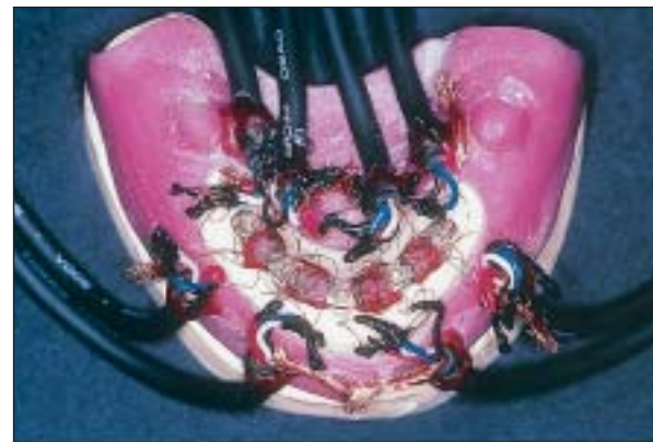
Fig 4b Assessment of framework deformation in a specimen with the assembled strain gauges.
