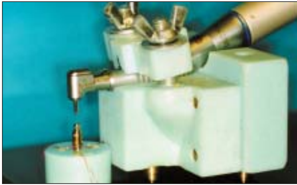
Fig 1 The experimental rig showing the mounting for the handpiece, vertical slides, and the implant body and abutment with the gold cylinder and screw in place.
