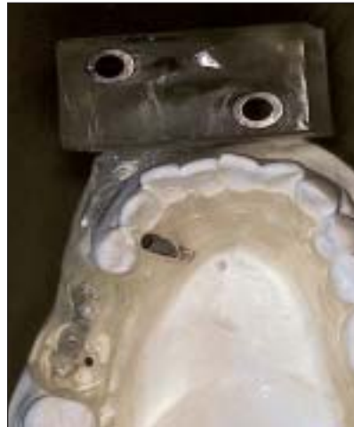
Fig 1a (Left) An acrylic resin cube, which includes 2 precisely positioned tubes made of titanium, is used to make a link between the planning software and the drilling machine.
