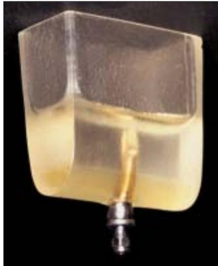
**Fig 2a** (Left) Photoelastic model of the grafted posterior maxilla with an implant.
