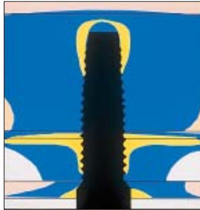
**Figs 10a and 10b** Stresses produced in model under 13.6-kg axial load when the stiffness of the simulated graft increased to its highest level. (Left) Isochromatic fringe patterns; (right) diagrammatic representations of stress intensities.
