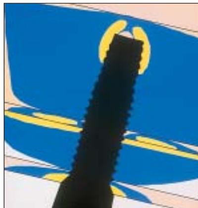
**Figs 11a and 11b** Stresses produced in model under 13.6-kg inclined load when the stiffness of the simulated graft increased to its highest level. (Left) Isochromatic fringe patterns; (right) diagrammatic representations of stress intensities.
