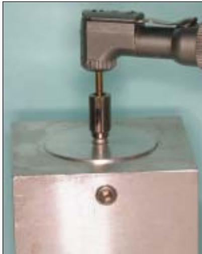
Fig 1 Tightening of abutment screw to 32 Ncm after implant/Procera abutment sample is placed in a holding device to ensure solid fixation.
