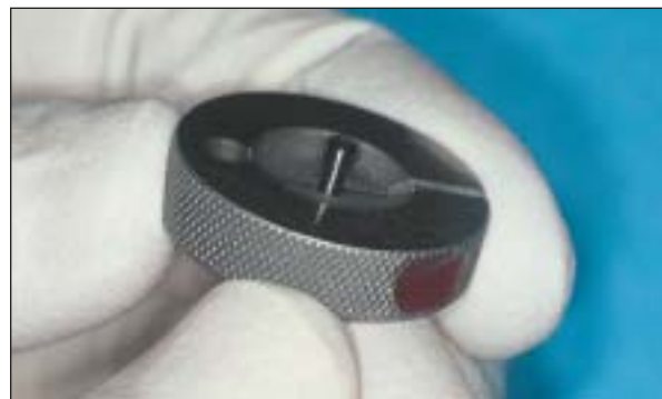
Fig 5b The abutment screw is placed inside the go/no-go gauge.
