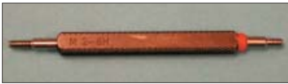
Fig 4a The go/no-go gauge that was used to determine the thread designation of the implant bore.
