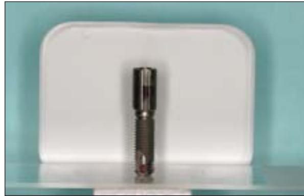
Fig 2 Positioning of the abutment-implant complex for radiographic assessment. Photograph demonstrates the angle of the radiographic source. The camera lens is positioned as if it were the head of the radiographic tube. The reference marker ( black ) located opposite one of the flat surfaces of the internal hexagons on the outer aspect of the Procera abutment was oriented perpendicular to the axis of the radiographic source.
