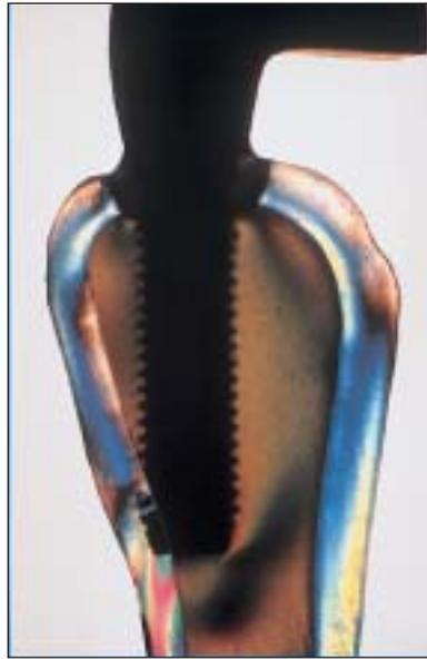
**Fig 7** (Left) Stress produced in model with implant engaging lingual cortical plate simulant having peri-implant defect under a 15-lb vertical load and 5-mm buccal cantilever.
