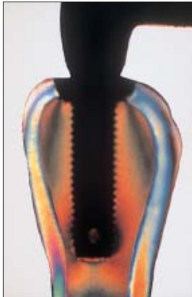
**Fig 6a (Left)** Stress produced in model with centrally placed implant having peri-implant defect under 15-lb vertical load and 5-mm buccal cantilever.
