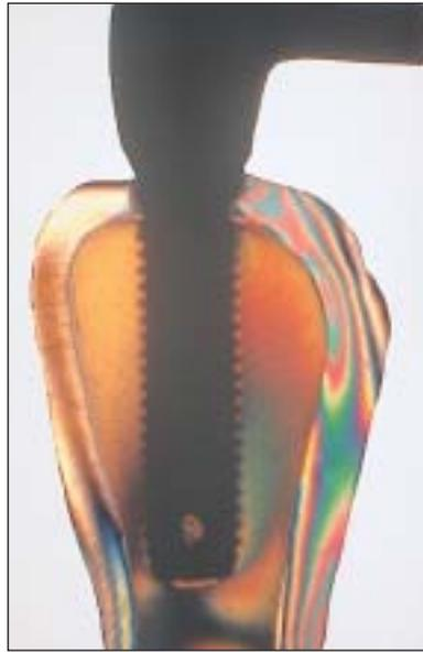
**Figs 3a (Left) and 3b (Right)** Stress produced in model with centrally placed implant and no peri-implant defect under a 15-lb vertical load. (Left) Three-millimeter buccal cantilever; (right) 5-mm buccal cantilever.
