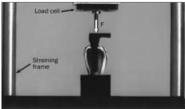
**Fig 1b** Model under load in straining frame.
