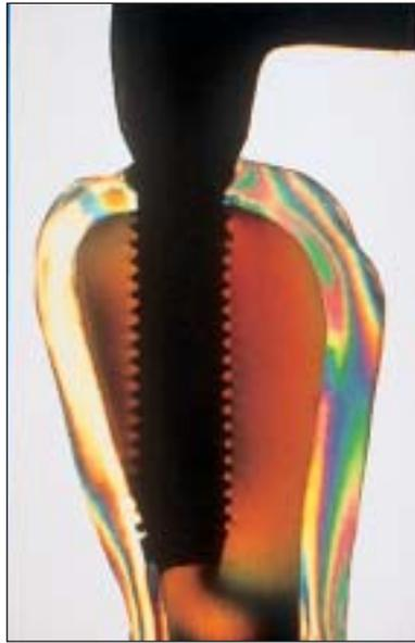
**Figs 5a (Left) and 5b (Right)** Stress produced in model with implant engaging lingual cortical plate simulant and no peri-implant defect under a 15-lb vertical load. (Left) Three-millimeter buccal cantilever; (right) 5-mm buccal cantilever.
