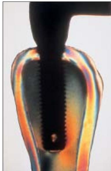
**Fig 2** (Right) Stress produced in model with centrally placed implant and no peri-implant defect under a 15-lb vertical load along implant axis.
