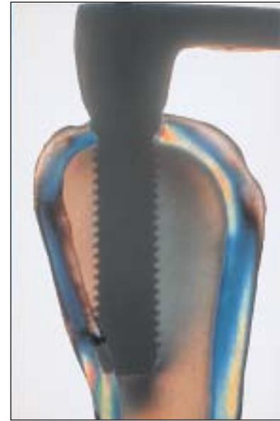
**Fig 4** Stress produced in model with implant engaging lingual cortical plate simulant and no peri-implant defect under a 15-lb vertical load.
