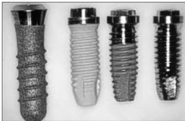
Fig 2 Dental implant surfaces used in this experiment. (Left to right) Titanium plasma-sprayed, hydroxyapatite, machined surface on first 3 threads and acid-etched surface on the other threads, and commercially pure titanium.
