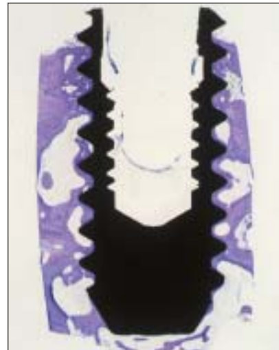
Fig 4c Test sample from a mandible. Note the bone trabeculae formed along the implant surface.
